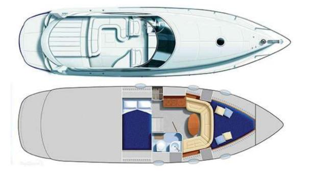
Shipyard: Pershing Model: Pershing 37 Lenght: 11,30 mt Beam: 3,25 mt Cabins: 2 + 1 toilet Guest Capacity: 8 people Crew: 1 Engines: 2 x 750 HP CAT Fuel consuption: 120 lt/h Cruising Speed: 25 knots Max Speed: 35 knots
